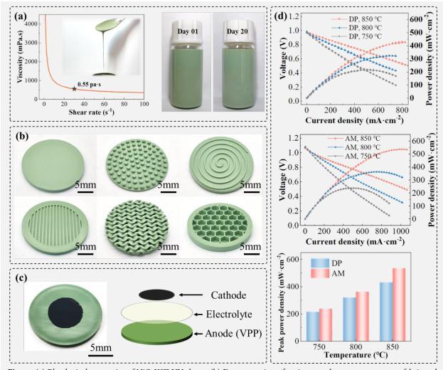
**Figure:** (a) Rheological properties of NiO-YSZ UV slurry. (b) Demonstration of various anode support structures fabricated by VPP. (c) NiO-YSZ anode-supported SOFC. (d) Comparison of the electrochemical performance between the 3D printed SOFC (AM sample) and the SOFC fabricated by the conventional dry pressing (DP) method.
