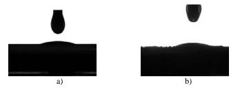
Fig. 7 HFE 7200 droplet on a) bare chip b) 4µm nanowire surface
