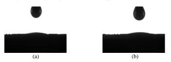
**Fig. 8** Droplet of 10 vol% mixture of a) HFE 7200 – Ethoxybutane b) HFE 7200 – Methanol, on  $4\mu m$  nanowire surface
