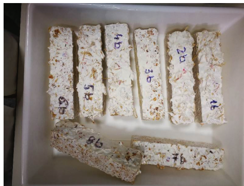
Figure 2: Material specimens of hemp mycelium composite (HMC) and wood mycelium composites (WMC)
