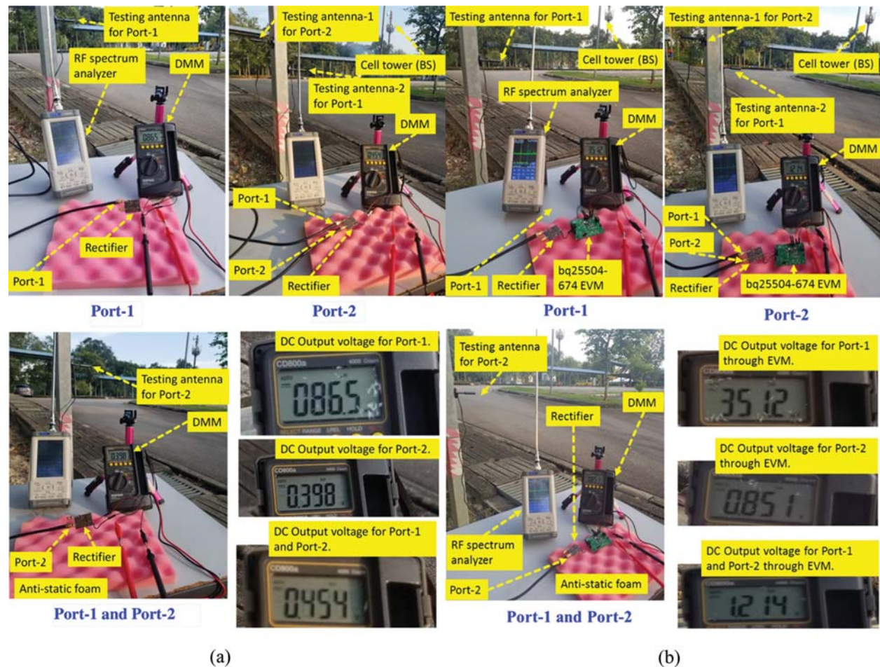
Figure 10: Proposed rectifier ambient measurement setups: (a) Ambiance only with bq25504-674 (b) Ambiance with bq25504-674
