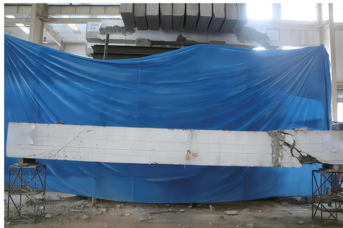
(b) Experimental photograph showing visible cracks, spalling, and reinforcement yielding.
