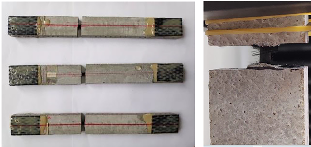
Figure 8: Failure mode observed in pull out tests with 30 mm embedded length. Adapted with permission from Ref. [48]. Copyright ©2021, Elsevier.
