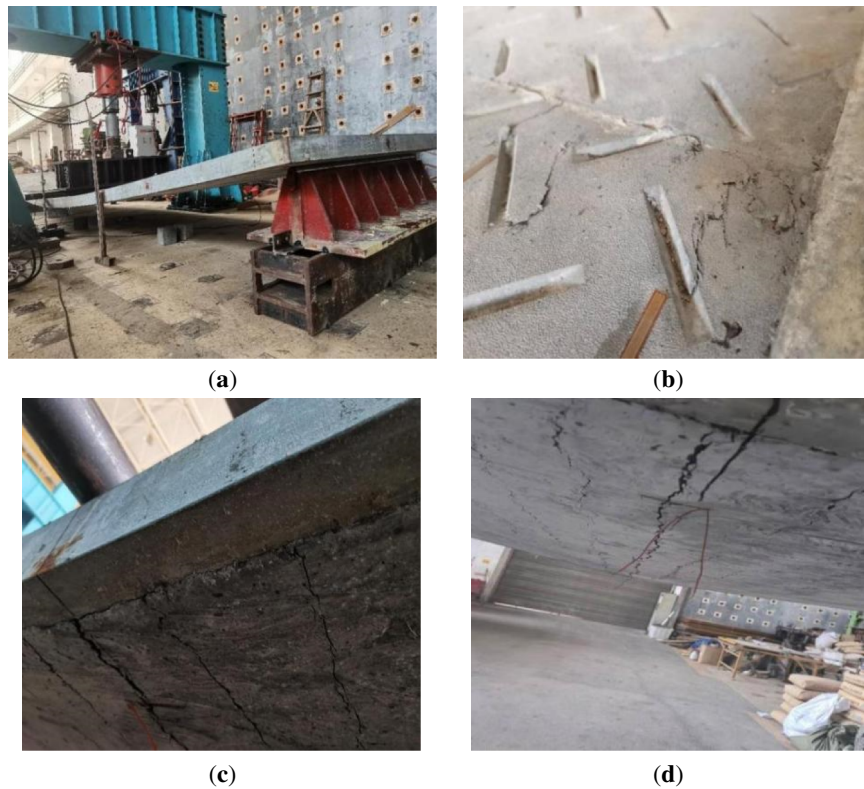
Figure 9: Failure mode diagrams: (a) overall bending and deflection of the UHPC slab; (b) compressive cracks at the top of the mid-span section; (c) cracks at the slab bottom edge; (d) primary crack at slab bottom.
