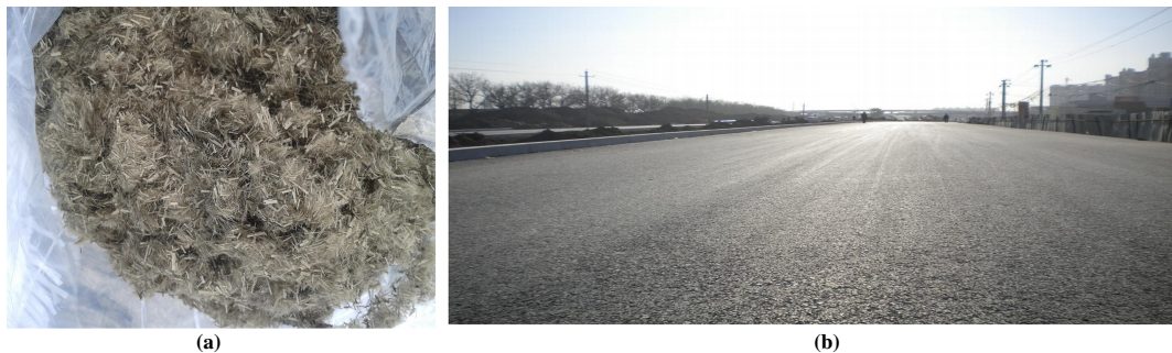
Figure 2: Applications of basalt short-cut fibers in asphalt pavement Construction (a) Basalt short-cut fibers, (b) Constructed asphalt pavement.
