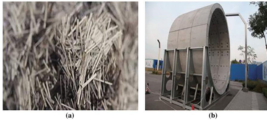
Figure 5: BF reinforcement in cement and shield tunnel segments (a) Short-cut BF for cement, (b) Basalt shield tunnel segments.
