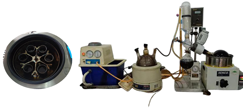
Figure 1: Extraction and distillation apparatus for aged asphalt binder.
