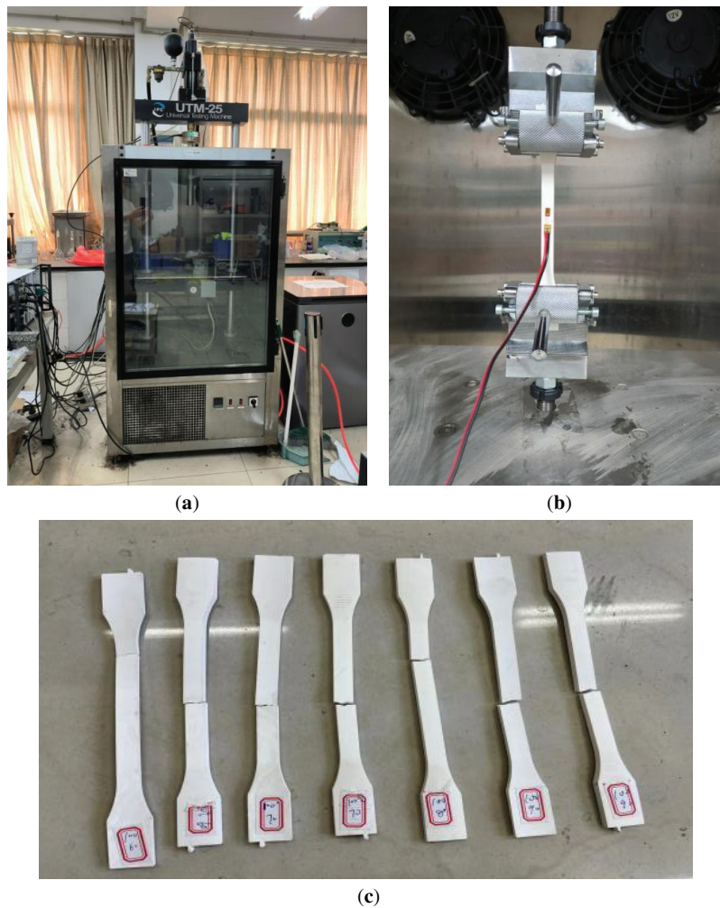
Figure 2: Loading system and specimens. (a) Loading system; (b) Specimen inside temperature chamber; (c) Specimens after fracture.
