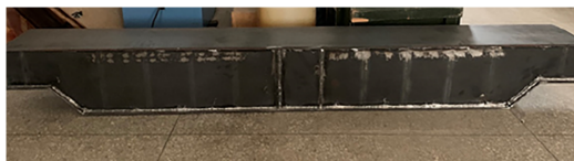
Figure 8: Physical picture of the main girder model.
