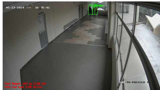
Figure 16: Annotated frame from Hallway 1 (camera code: 13H-PA-PASILLO 1), with three occupants detected and a computed load of 0.08 \text{ kN/m}^2 .
