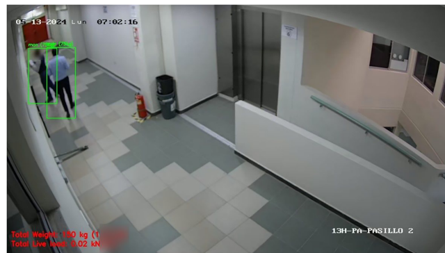
Figure 19: Annotated frame from Hallway 2 (camera code: 13H-PA-PASILLO 2), with three detected individuals and a computed load of 0.02 \text{ kN/m}^2 .
