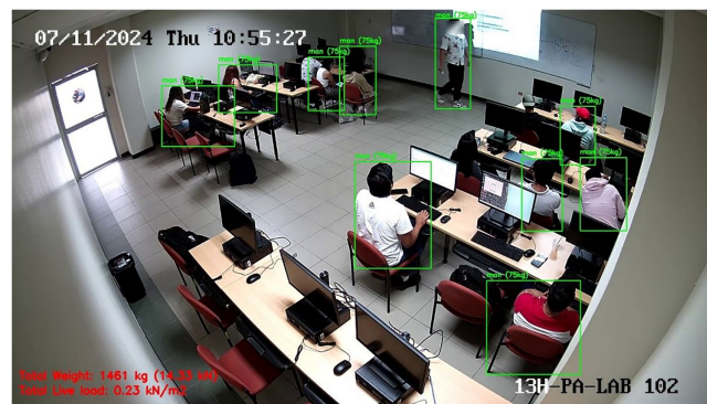
Figure 13: Annotated frame from Computer Laboratory 2 (camera code: 13H-PA-LABORATORIO 2), showing ten detected individuals with a computed total load of 1461 kg including furniture load (0.23 kN/m 2 ).
