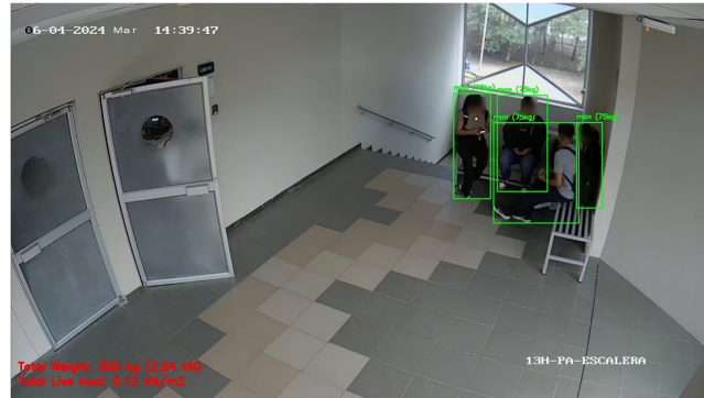
Figure 22: Annotated frame from the Stairwell Connector (camera code: 13H-PA-ESCALERA), showing four detected individuals and a computed load of 0.12 \text{ kN/m}^2 .
