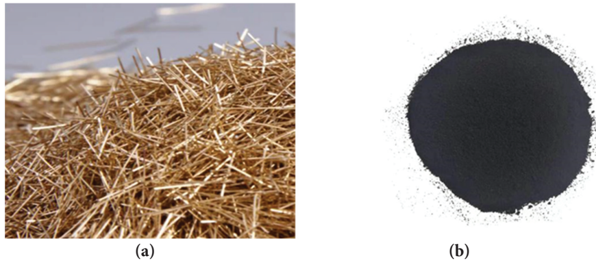
Figure 1: Morphology of materials: (a) Steel fibers; (b) Recycled rubber powder.
