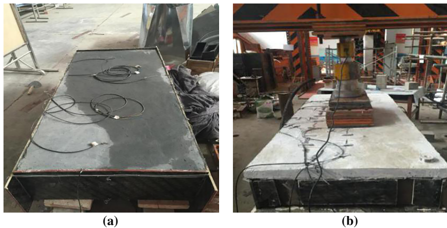
Figure 12: (a) RPC surface after conservation; (b) Load test of model.
