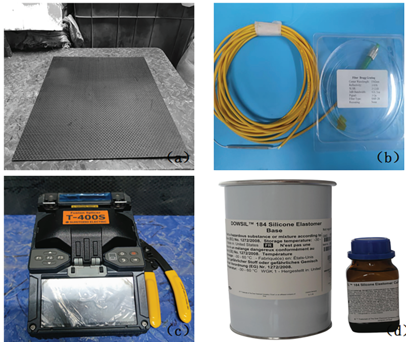
Figure 3: Items required for making the FBG sensor array: (a) CFRP laminates; (b) FBG sensors; (c) T-400S optical fiber fusion splicer; (d) SYLGARD™184 silicone elastomer
