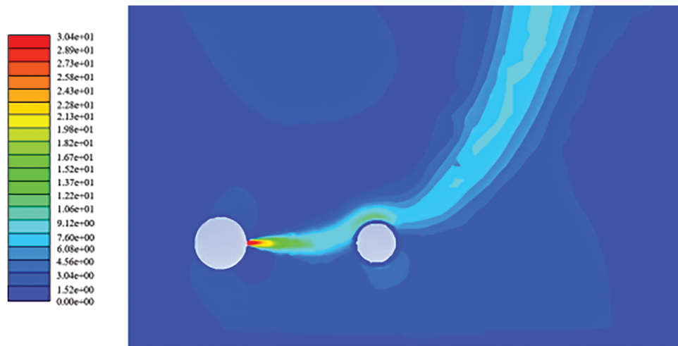
Figure 7: Cloud view of natural gas combustion velocity field at the leakage vent
