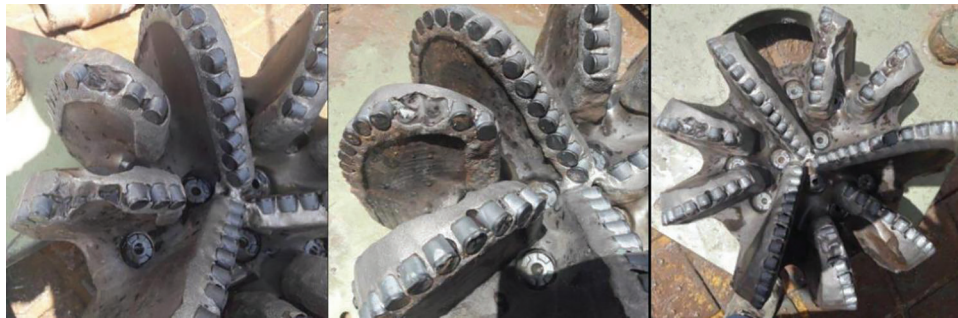
Figure 6: Images show the wear of the used PDC drill bit in Well-1
