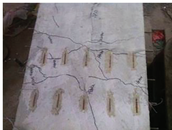
Figure 8: Transverse cracks in the negative moment
