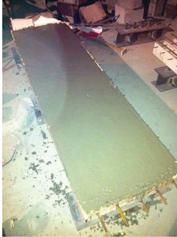
Figure 5: Test specimen manufacture
