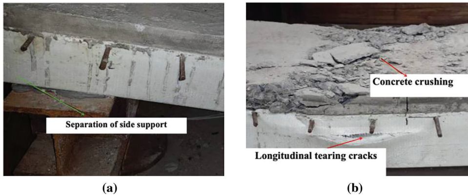
Figure 9: Local failure of specimen GC-1. (a) Resin layer debonding at the side support. (b) Longitudinal tearing of GFRP profile web
