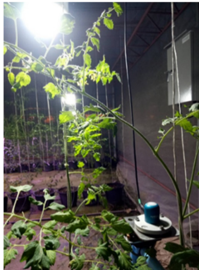
Figure 4: Light intensity sensor in the greenhouse.
