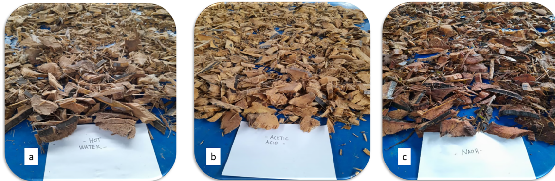
Figure 2: OPT particles of different pre-treatments (a) hot water, (b) acetic acid and (c) NaOH
