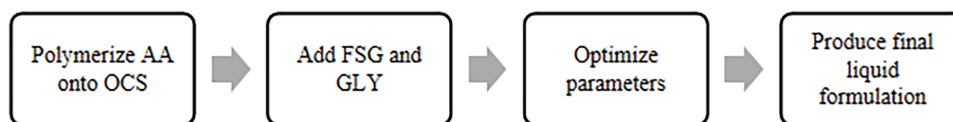
Figure 12: Processing steps involved in the fabrication of OCS-g-PAA/FSG/GLY liquid dust suppressant through graft polymerization and hydrogen bonding for eco-friendly dust control applications
