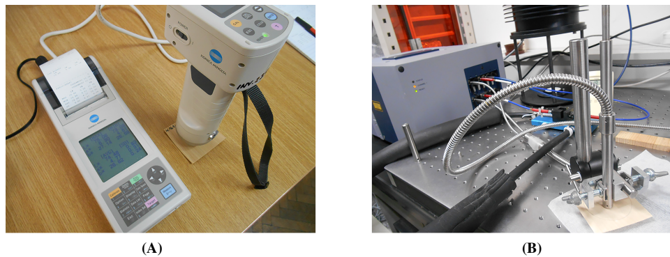
Figure 1: Colour and NIR measurement. (A) Konica Minolta CR-400 Chroma Meter. (B) Matrix-F FT-NIR spectrometer (Bruker Optics)
