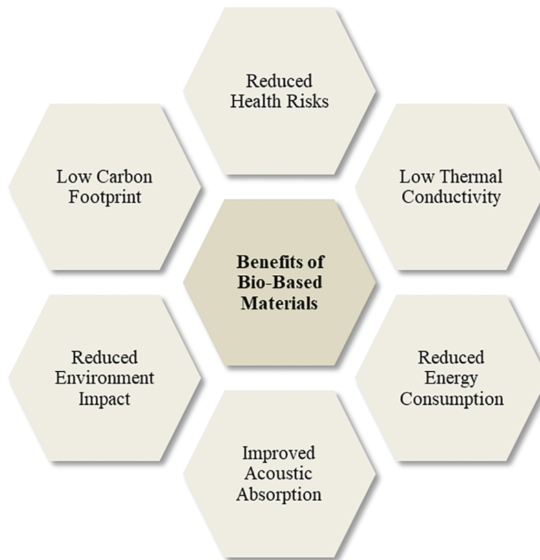
Figure 4: Schematic illustration outlining some of the key benefits provided by thermal insulation boards manufactured from bio-based materials
