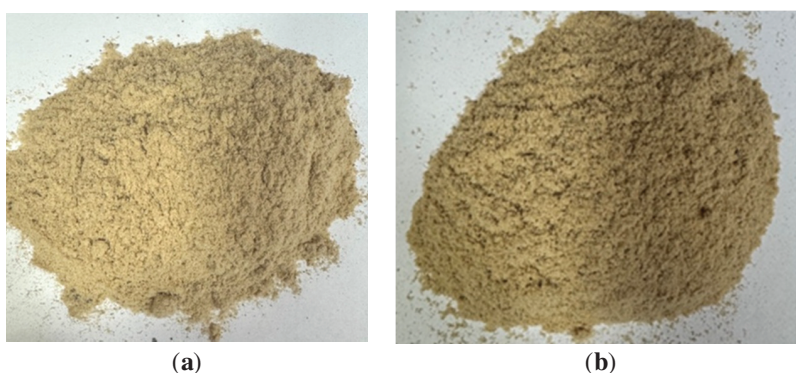
Figure 1: Samples of fillers: (a) untreated; (b) ozonation for 120 min, ozone concentration 40 mg/L, temperature 40°C
