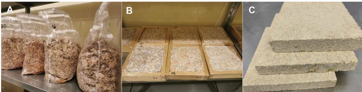
Figure 1: Development stages of EPW mycelium biocomposites: (A) initial cultivation in filter patch bags; (B) secondary growth in molds; (C) final biocomposite panels
