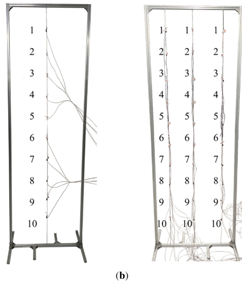
Figure 4: Schematic design and sensor layout of the rack temperature measurement frames. (a) Schematic diagram of the temperature measurement point layout for the server rack inlet and outlet; (b) Photograph of the physical measurement frames with actual thermocouple installation.
