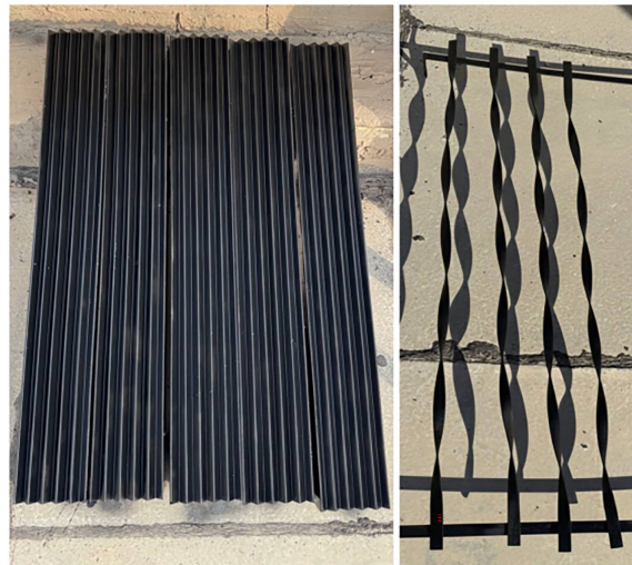
Figure 2: Corrugated air ducts with twisted tapes configurations.
