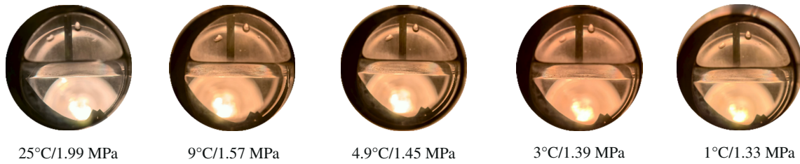
Figure 6: Observation diagram of the experimental process at 50% water content + single CO 2 (P = 2 MPa).
