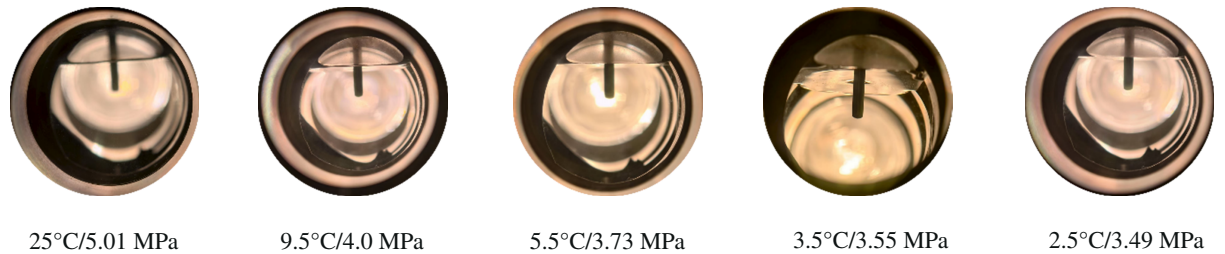
Figure 4: Observation diagram of the experimental process at 70% water content + single CO 2 (P = 5 MPa).
