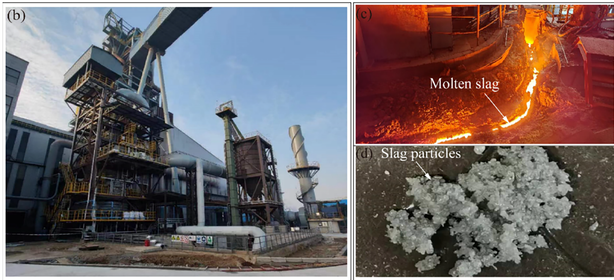
Figure 2: The blast-furnace slag waste-heat-recovery system. (a) The technology scheme for 60 t/h blast furnace slag disposal. (b) The industrial project. (c) The molten blast furnace slag. (d) The slag particles after treatment [43].
