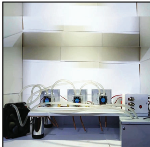
Figure 7: Device from inside showing copper tubes
