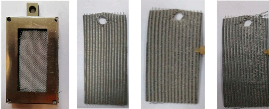
Figure 10: Screen mesh sample of metal mesh screen with solid mass fraction of 0.5% and liquid velocity 2 m/s.
