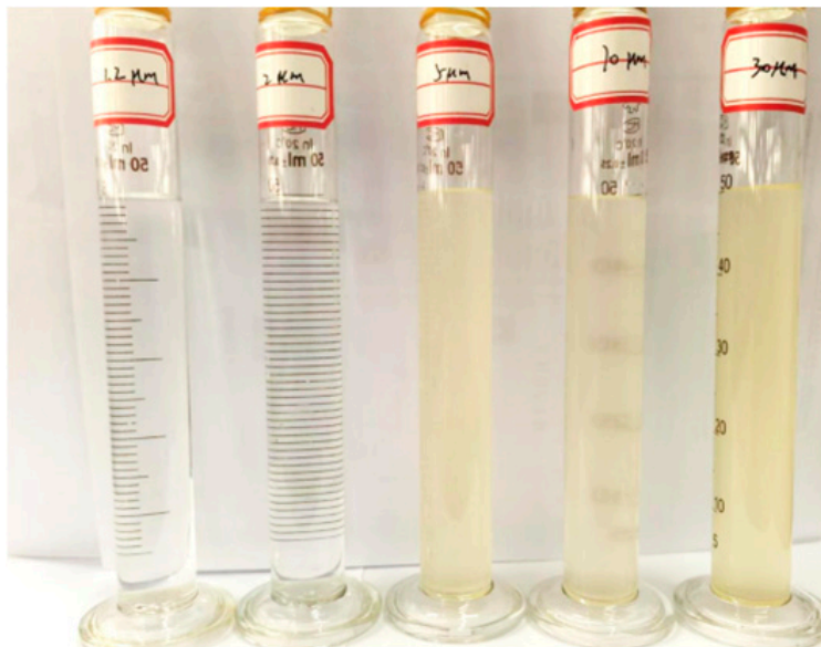
Figure 5: Filtrates obtained using membranes with different pore sizes.
