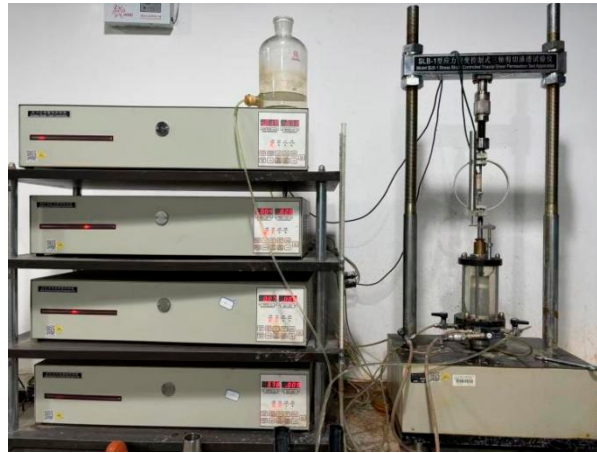
Figure 2: SLB-1 triaxial seepage-shear apparatus used in this study.
