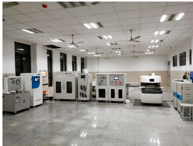
Figure 3: Online nuclear magnetic resonance displacement experimental apparatus.
