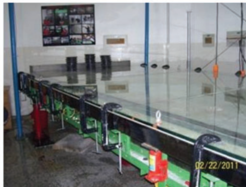
Figure 6: Model of dynamic water grouting and the experimental setup used (a, b). Adapted with permission from Ref. [77]. Copyright © 2016, CSRME Publishing
