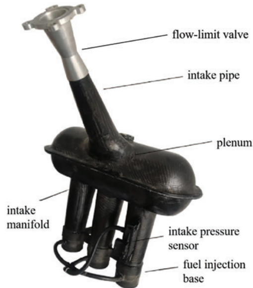
Figure 1: Structure diagram of engine air intake system with flow-limit valve
