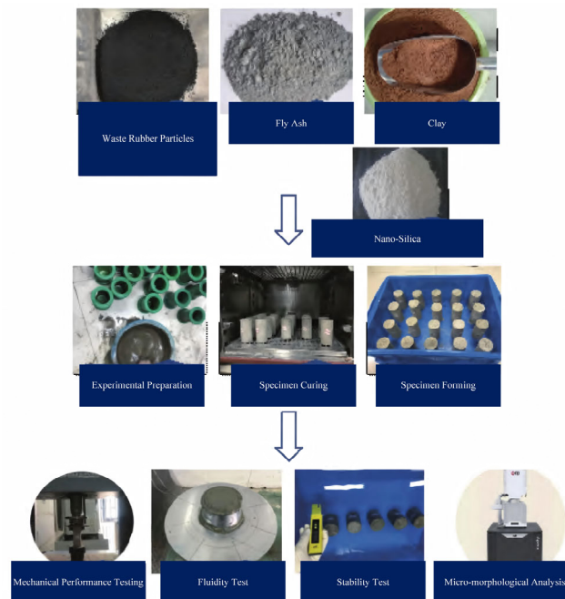
Figure 11: Test process of solid waste grouting materials. Adapted with permission from Ref. [102]. Copyright © 2023, Coal Sci Technol.
