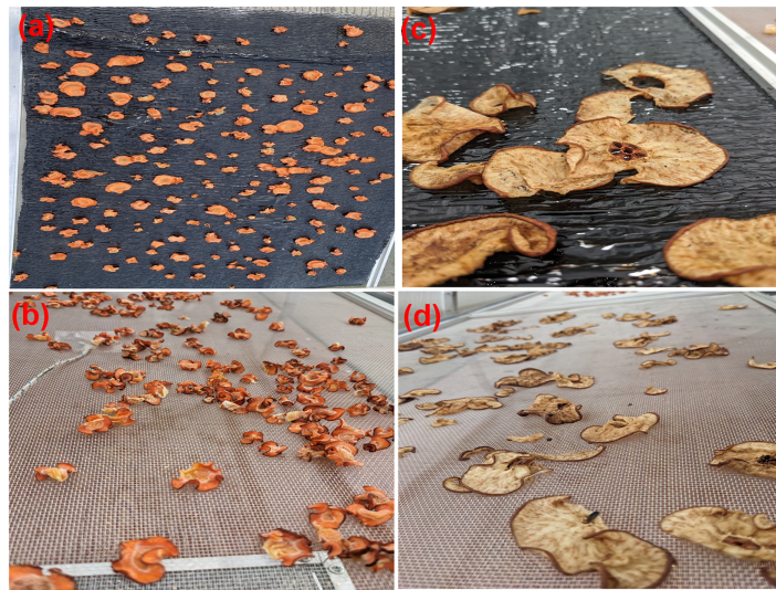
Figure 2: Experimental results after 20 days for (a) a selective absorber-coated tray with carrots, (b) a non-selective absorber-coated tray with carrots, (c) a selective absorber-coated tray with pears and (d) a non-selective absorber-coated tray with pears.
