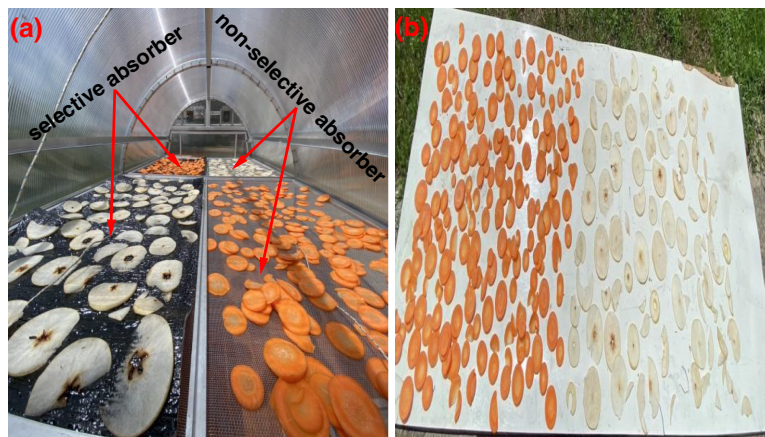
Figure 1: Experimental view of (a) the solar dome inner view with a selective and non-selective absorber-coated tray. All the trays are equipped with 600 g of carrots and 600 g of pears, separately. (b) 600 g of carrots and pears are placed for conventional sun/open drying.
