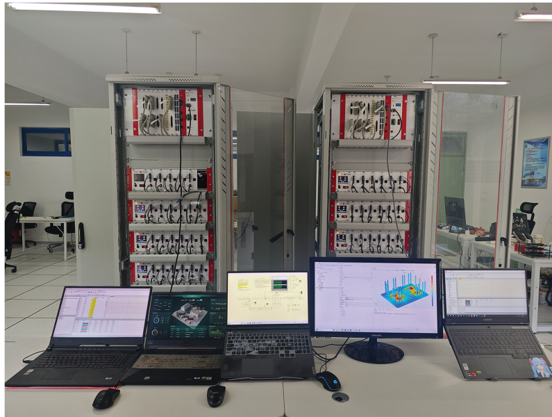
Figure 4: MMC-UPFC prototype photograph
