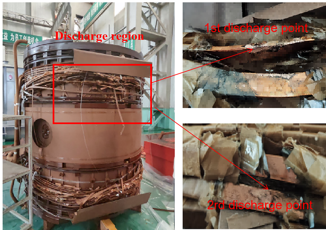
Figure 13: Location of the interturn short circuit fault.
