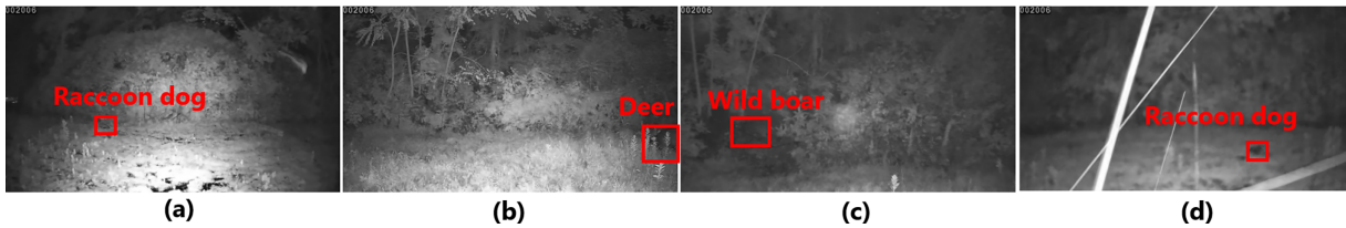
Figure 8: Example images of missed detections caused by (a) small target size, (b) partial visibility, (c) low contrast with the background, and (d) image blur.
