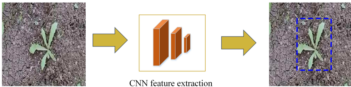
Figure 9: Schematic diagram of the one-stage object detection framework. The figure illustrates how one-stage detectors perform feature extraction, classification, and bounding box regression within a unified network.
