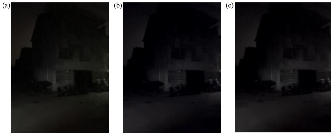
Figure 6: Comparison of denoising effects for low-illumination high-noise urban scenes. (a) Noisy input image; (b) Dual-branch model without FDPL; (c) Dual-branch model with FDPL in this paper.
