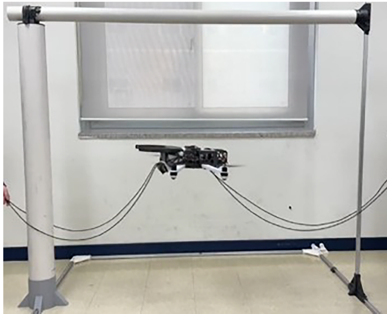
Figure 4: A snapshot with hardware prototype of resting UAV.
