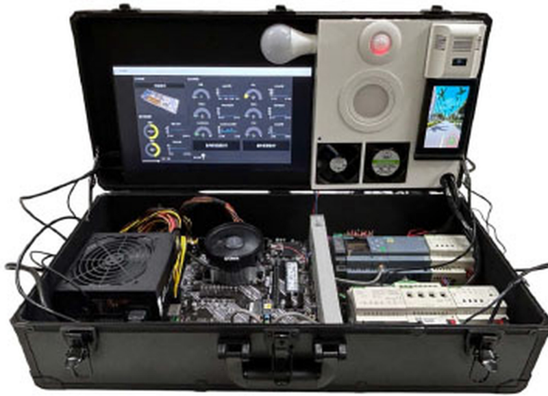
Figure 5: Physical digital twin box replicating the real building electrical control system. The digital twin box is designed to be structurally and functionally identical to the on-site electrical cabinet, enabling real-time data synchronization and historical data replay for analysis and validation.
