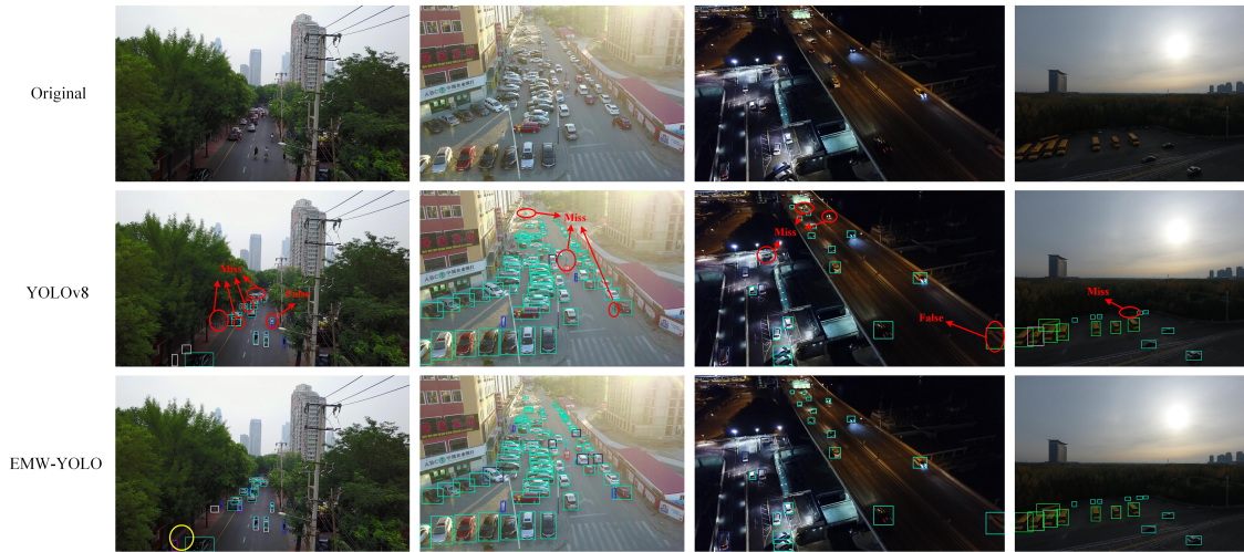
Figure 9: Comprehensive detection performance comparison between YOLOv8 and EMW-YOLO in extremely complex scenarios. These diagrams include four major complex scenes: large shooting angles (the first column), dense distribution (the second column), low illumination (the third column) and overexposure (the fourth column).
