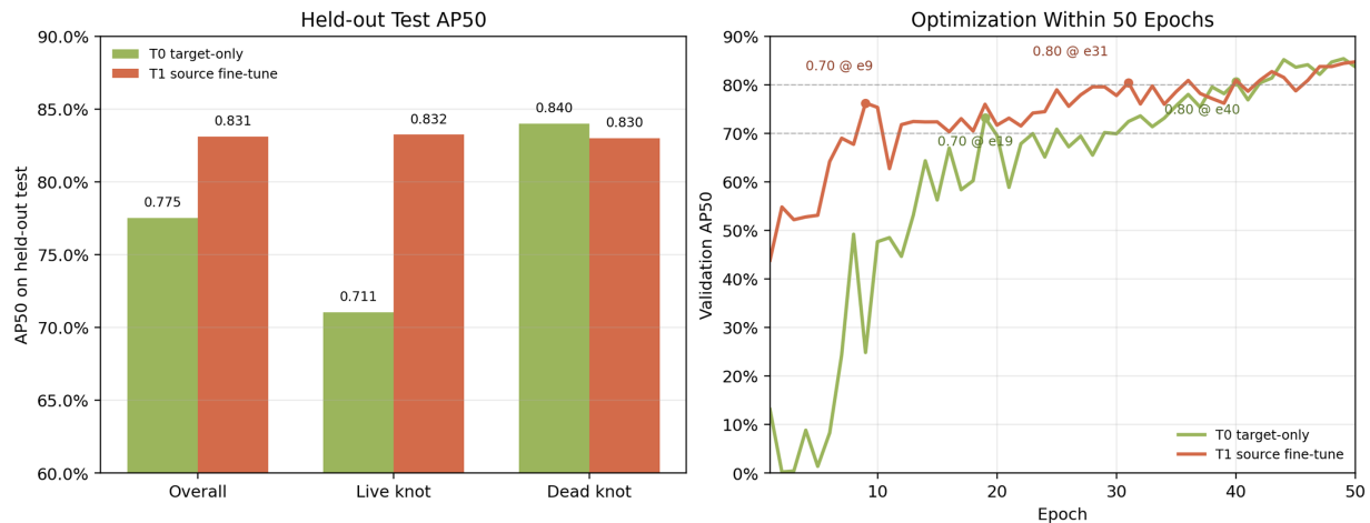
Figure 4: VNWoodKnot adaptation under 50-epoch budget. Left: held-out test AP50 overall and by class for target-only training and curated-benchmark source fine-tuning. Right: validation AP50 trajectories for the first 50 epochs.
