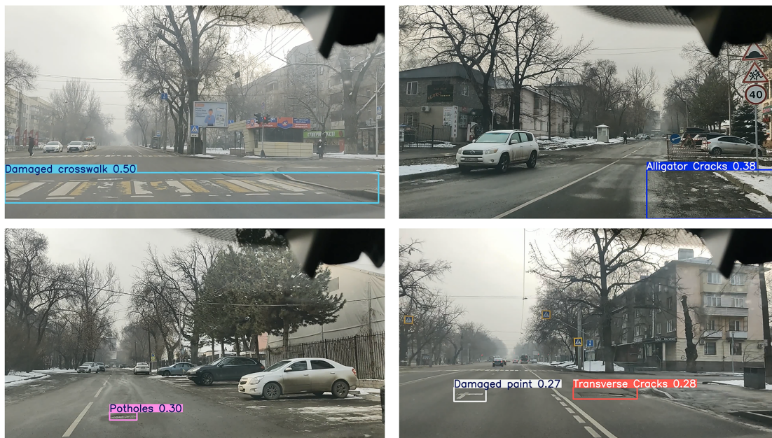
Figure 12: Real-time crack detection.
