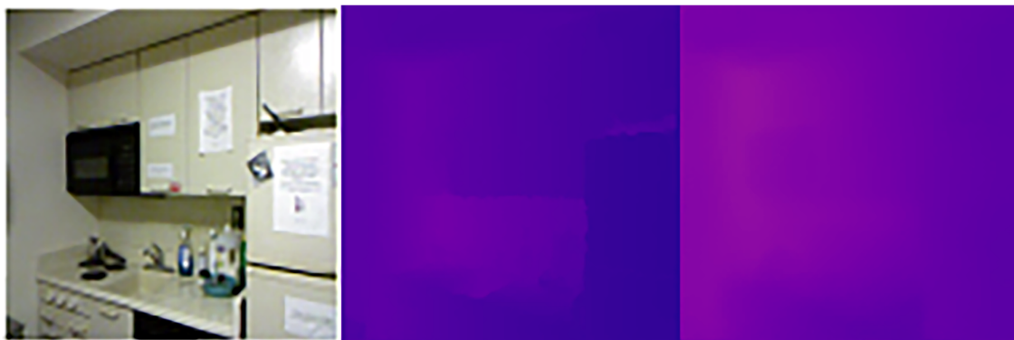
Figure 8: Failure cases on NYU Depth v2 for the auxiliary multi-scale + SI-Log variant, showing over-regularised (oversmoothed) predictions in challenging regions. Larger depths are brighter, smaller depths are darker.
