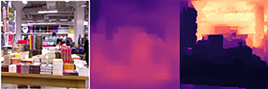
Figure 9: Failure case qualitative example on NYU Depth v2 for the final DeepEchoNet model (selected by per-image RMSE). From left to right: RGB input, DeepEchoNet prediction, and ground-truth depth. Depth maps are clamped to a fixed range, linearly normalised to [0,1] , and visualised with a perceptually-uniform sequential colormap (larger depths are brighter).
