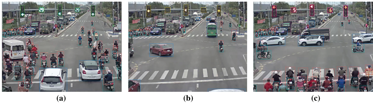
Figure 3: Representative examples of traffic-light annotations in the proposed dataset. (a) Illustrates a green traffic signal, including the remaining movement time and the corresponding permitted movement direction. (b) Shows a yellow traffic signal. (c) Presents a red traffic signal displaying a countdown timer indicating the remaining waiting time.
